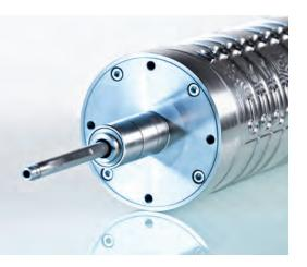
The Wink AirTec system consists of rotary dies with a compressed air connection. The cut-out waste can be blown via air passage holes positioned around the cylinder, directly into the extraction unit which is attached to the vacuum system. This procedure guarantees that no waste is left stuck in the cylinder cavities or in web.
